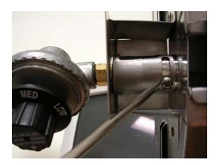
To adjust for proper flame, use a Philips screw driver to loosen screw. Turn clockwise to close the air shutter, and counterclockwise to open. After adjusting, tighten screw to fix air shutter.
